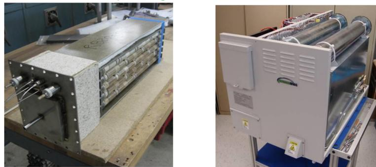
**Cell testing:** The Acumentrics tubular cell is conducive to experimental designs magnifying defect degradation. Miniature cells incorporating the defect can be fired so that areal degradation effects are exaggerated relative to a full size cell. The cell tests can be conducted with reference cells to distinguish degradation caused by the flaw from materials degradation.
